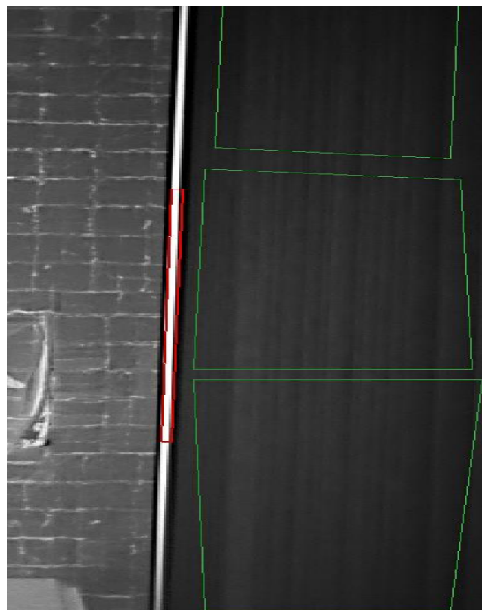
Figure 10. Hot Tube with Red Alarm Box
